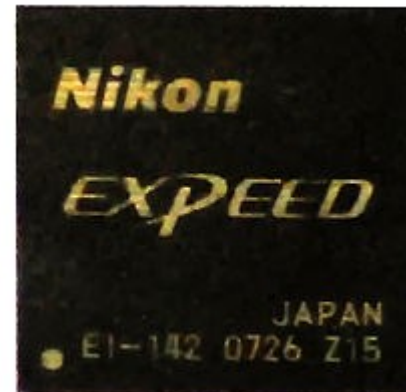
Nikon EXPEED, a system on a chip including an image processor, video processor, digital signal processor (DSP) and a 32-bit microcontroller controlling the chip
